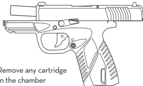
**Fig. 6.** Remove any cartridge in the chamber
