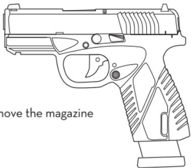
**Fig. 5.** Remove the magazine
