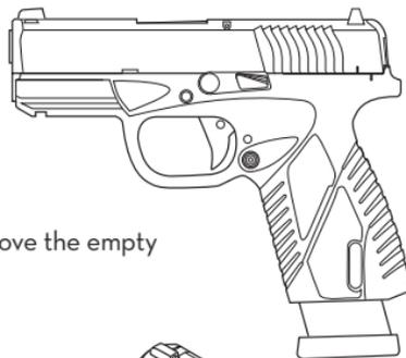
**Fig. 10.** Remove the empty magazine
