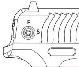
**Fig. 1 - internal locking system in fire position**
