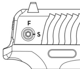
**Fig. 1 - internal locking system in locked position**
